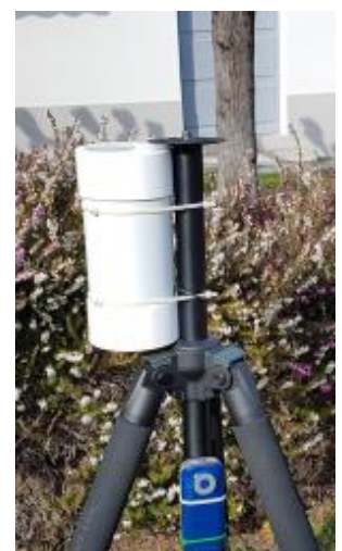
Ninox field of view not obstructed by the top of the tripod
