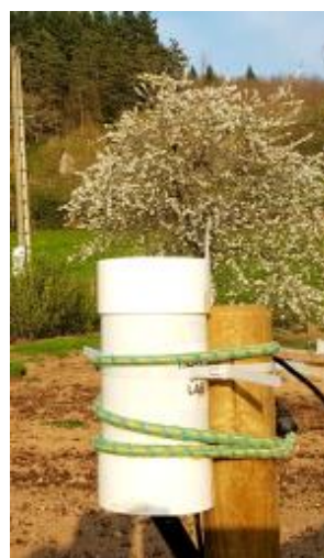
Ninox far from any obstacle that could obstruct its field of view
