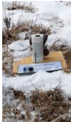
Too close from the ground with the risk that humidity goes into the tube
